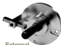
External skiving tool with one external tool
